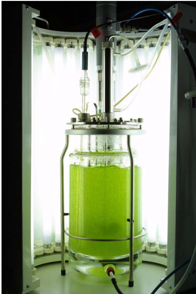
Figure 25. This type of bioreactor is used to grow Physcomitrella patens for human proteins and human blood-clotting factor IX. Photo by Ralf Reski.
