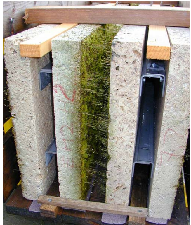
Figure 4. These mosses are being cultured on tufa to be used in building construction. Photo by Michel Chiaffredo.
