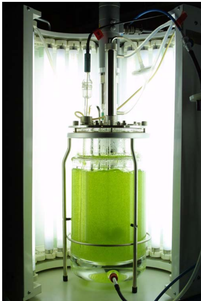
Figure 28. Moss bioreactors provide sterile cultures of Physcomitrella patens , avoiding the contamination problem prevalent with soil-grown plants. Photo by Ralf Reski.
