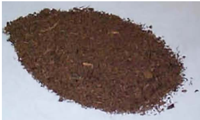
Figure 3. This pile of Hydro-Weed, made with Sphagnum , is a good absorbent of oil while repelling water. Photo from Hydro-Weed website.
