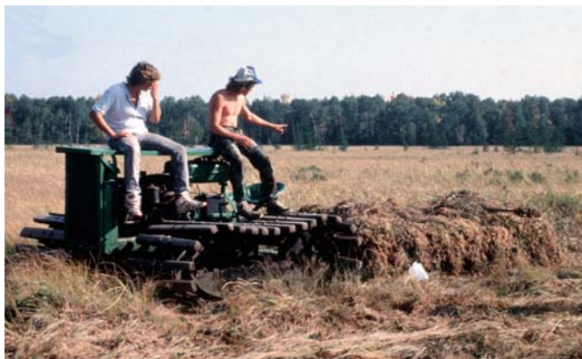
Figure 7. A tractor with a wooden tread pulls the wagon on which peat is loaded, minimizing damage to the peatland. Photo by Janice Glime.
