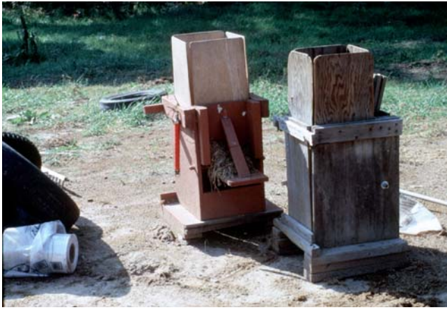
Figure 11. This packaging equipment is used for bagging the dry mosses ready for sale without need for a building or power. Photo by Janice Glime.
